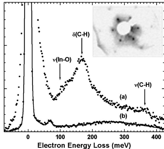
FIG. 4. The HREEL spectra (points) for a probing energy of 15 eV are shown (a) prior to and (b) after AHC. Surface contaminant vibrational modes are present in (a), whilst these contaminant modes are absent after AHC (b). The clean surface spectrum in (b) is simulated by semiclassical dielectric theory (line). The inset shows the  $(1 \times 1)$  LEED pattern recorded after cleaning, using an electron energy of 164 eV.
