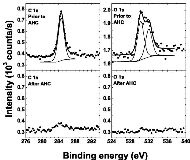
FIG. 1. The  $45^\circ$  TOA C 1s and O 1s core-level spectra (circles) recorded prior to and after AHC. For the prior to AHC spectra, for both the C 1s and O 1s, the corresponding fits (thick lines) are shown. The decomposed background and peak contributions of each fit (thin lines) are also shown vertically offset for all spectra.
