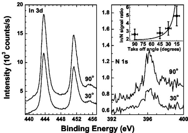
FIG. 3. The In  $3d$  and N  $1s$  core-level spectra after AHC, at both  $90^\circ$  and  $30^\circ$  TOA. The In/N intensity ratio determined from XPS against the angle is plotted in the inset. Also included in the inset is the calculated variation in the In/N photoelectron intensity ratio with angle, assuming an In-adlayer model analogous to GaN $\{0001\}$ - $(1 \times 1)$  surfaces.
