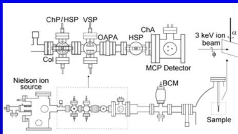
The experimental arrangement of the Warwick modular CAICISS apparatus (described in detail elsewhere<sup>1</sup>). The detector-to-sample separation is 80 cm. The scattering geometry adopted for the CAICISS experiments and the rotation axes for the incident polar ( $\alpha$ ) and azimuthal ( $\phi$ ) angles are shown in the upper-right of the image.
