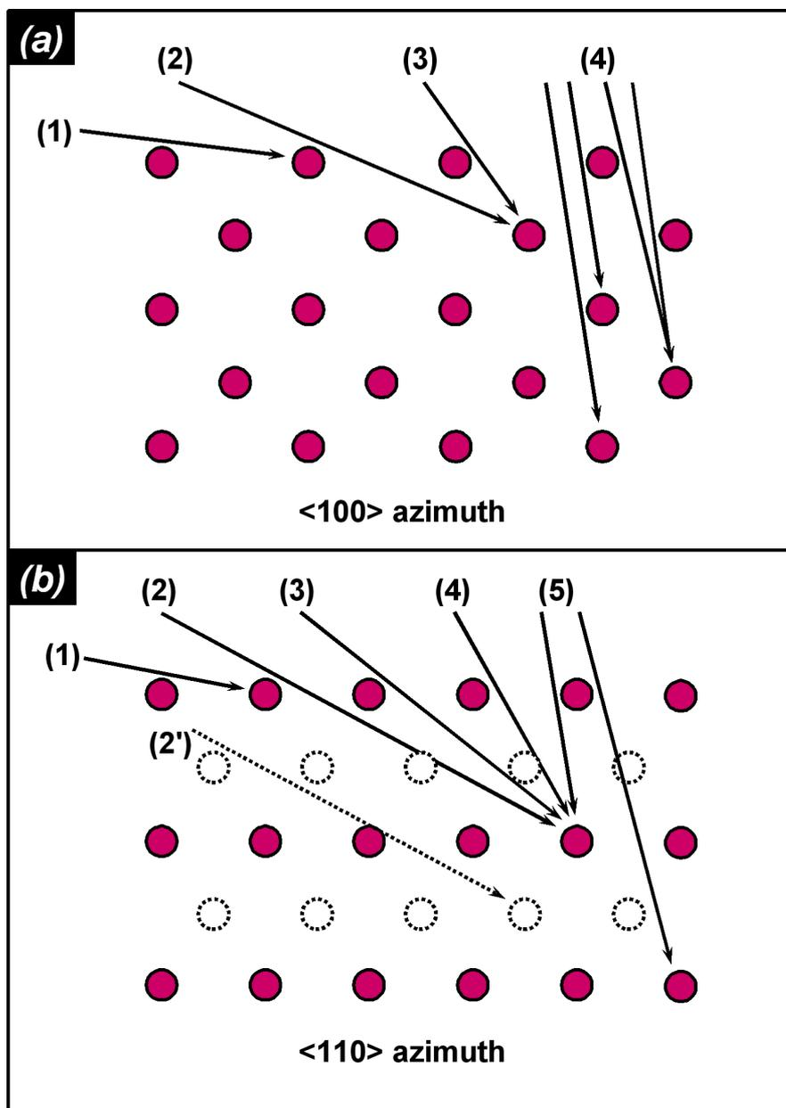
Figure 6.1: The scattering geometries which lead to peaks in the CAICISS spectra obtained in (a) the  $\langle 100 \rangle$  and (b) the  $\langle 110 \rangle$  azimuthal directions on the Cu(100) surface. This combination of azimuthal directions allows a full structural determination down to the fifth layer of the crystal. Atoms represented by dashed lines lie in different planes with respect to the incident ion beam.
