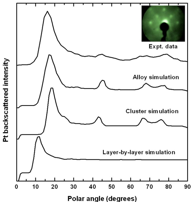
Figure 6.5: CAICISS data in the  $\langle 110 \rangle$  azimuth following the deposition of 0.55 ML of Pt on the Cu(100) surface. Also shown are the simulated profiles from three Pt growth models, which predict that an alloy in the surface region has been formed. The inset in the upper-right shows the  $c(2 \times 2)$  LEED pattern recorded at 130 eV from the surface.
