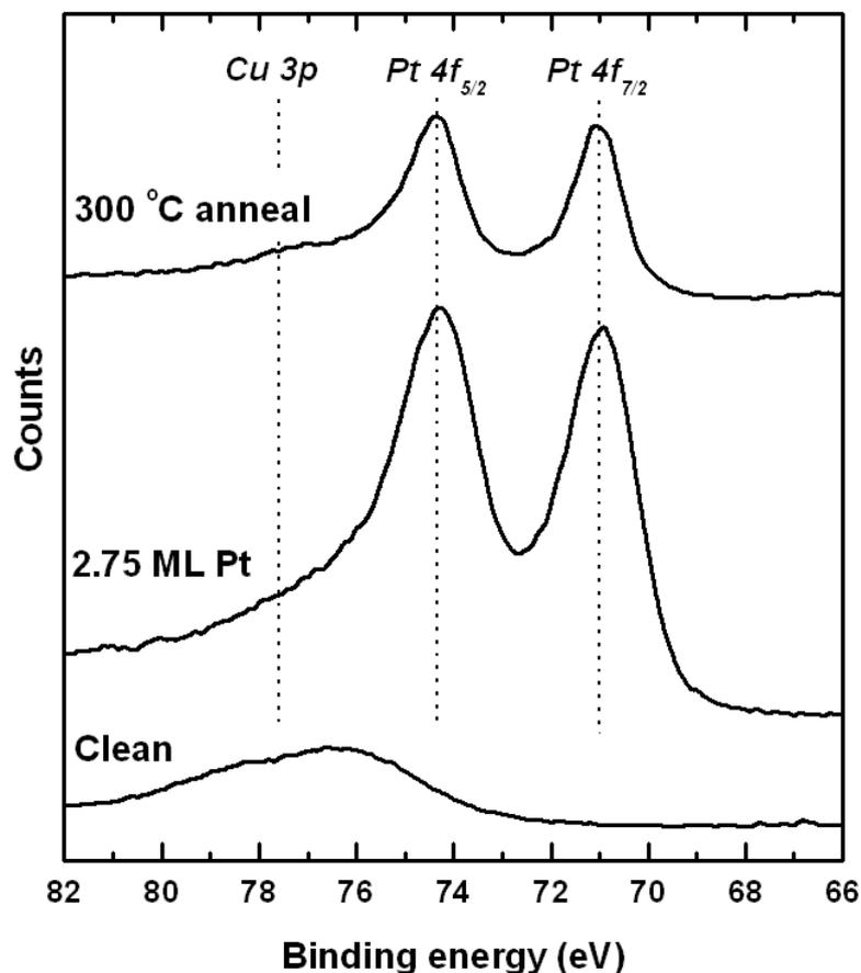
Figure 6.9: The Pt 4*f* and Cu 3*p* region of the XPS spectra taken from the surface at three stages of the investigation. The clean surface shows only the Mg K<sub>α</sub> Cu 3*p* peaks. At a Pt coverage of 2.75 ML, only the Pt 4*f* peaks were observed, with the Cu 3*p* peaks re-emerging following annealing at 300°C.
