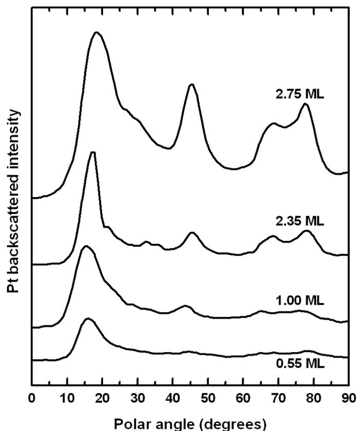
Figure 6.6: CAICISS Pt peak profile as a function of Pt coverage. Peaks corresponding to sub-surface Pt are present at sub-monolayer coverage suggesting the formation of an alloy on deposition. These peaks increase in intensity with further Pt deposition up to 2.75 ML.
