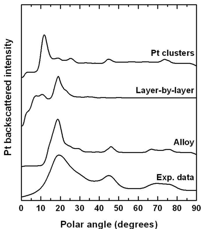
Figure 6.4: CAICISS data recorded in the  $\langle 110 \rangle$  azimuth following the deposition of 0.25 ML of Pt on the Cu(100) surface. Also shown are the simulated profiles from three Pt growth models (layer-by-layer growth of a Pt film, 3D Pt-island formation and Cu-Pt alloy formation in the surface region). The features within the experimental data appears to favour the Cu-Pt alloy model.
