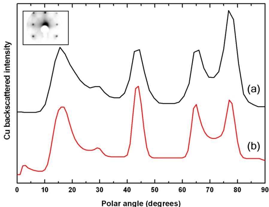
Figure 6.2: (a) CAICISS data from the clean Cu(100) surface in the  $\langle 110 \rangle$  azimuth, along with (b) the simulated profile for the derived structure outlined in the main text. The inset in the upper-left shows the inverse of the  $(1 \times 1)$  LEED pattern recorded at 64 eV prior to the CAICISS data being taken.
