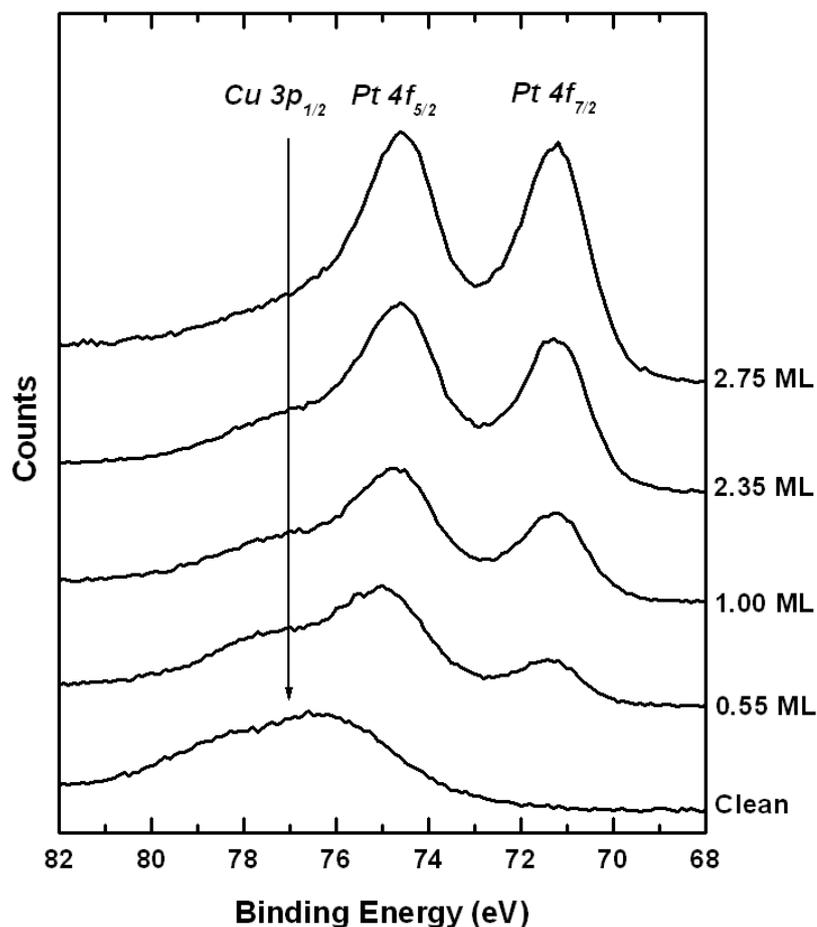
Figure 6.7: The Pt 4f (71.2 eV, 74.5 eV) and Cu 3p (75.2 eV, 77.5 eV) photoemission peaks from clean Cu(100) and during Pt deposition up to a coverage of 2.75 ML. All data were recorded at a take-off angle of 45°.
