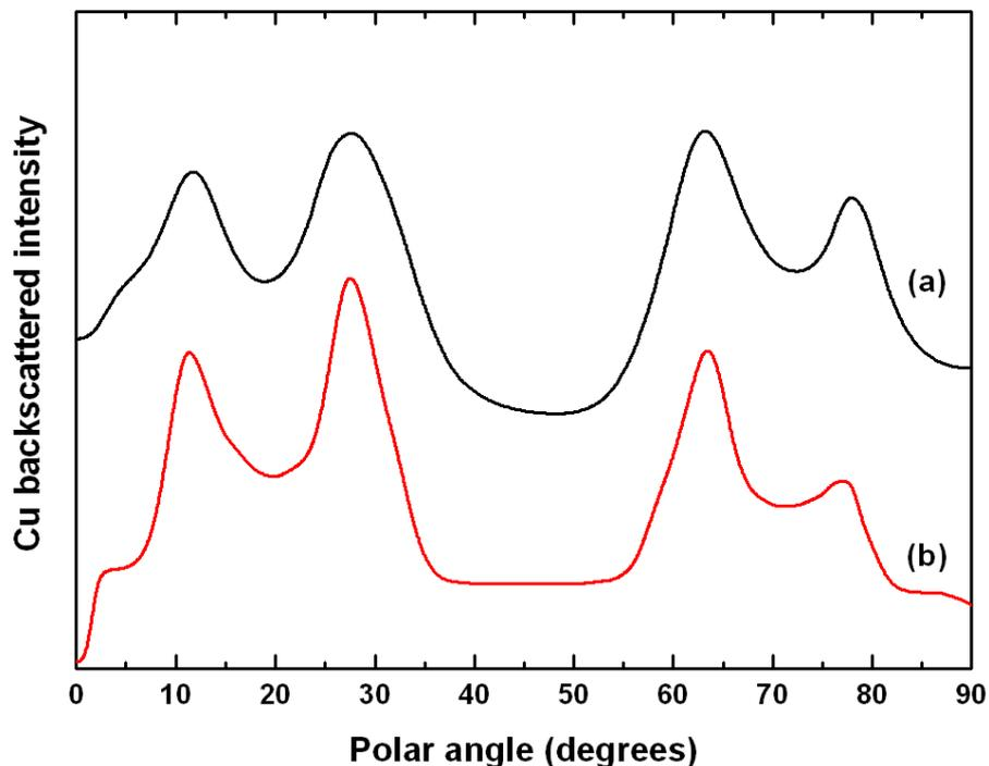
Figure 6.3: (a) CAICISS data from the clean Cu(100) surface in the  $\langle 100 \rangle$  azimuth, along with (b) the simulated profile for the derived structure outlined in the main text.
