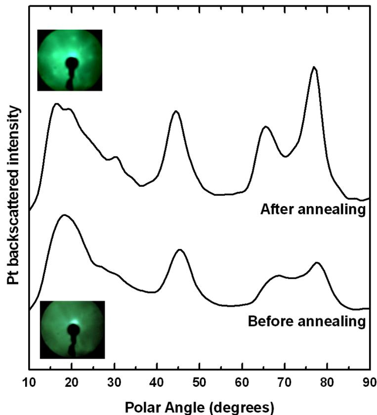
Figure 6.8: CAICISS and LEED observations from the surface with a Pt coverage of 2.75 ML prior to and following annealing at 300°C for 10 minutes. Both CAICISS and LEED show signs of some ordering at the surface caused by the annealing treatment. The increase of the intensities of the features at higher polar angles suggests that a significant proportion of the Pt at the surface has diffused into the sub-surface region during annealing. Both LEED patterns shown were recorded at 130 eV.
