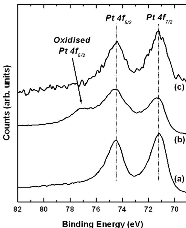
Figure 7.12: The Pt 4f region recorded from three different samples. (a) The data recorded from a clean Pt(111) surface. (b) The data collected following the oxidation of the Pt(111) surface (as detailed in chapter 5), showing an additional feature at 76.8 eV. (c) The Pt 4f region recorded following the deposition of 0.31 ML of Pt on the Ni(110) surface. Note the shoulder feature at 76.8 eV was not observed in the latter case.
