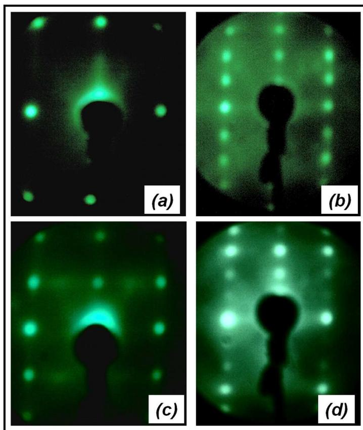
Figure 7.7: (a) The  $(1\times 1)$  LEED pattern recorded from the clean Ni(110) surface, along with (b) the  $(3\times 1)$ -O added row following an oxygen exposure of 1.0 L, (c) the  $(2\times 1)$ -O structure observed following exposure of 1.5 L and (d) the  $(3\times 1)$ -O missing row structure observed following a total exposure of 3.0 L. The clean surface LEED pattern was recorded at 78 eV, whilst the remaining patterns were recorded at 92 eV.
