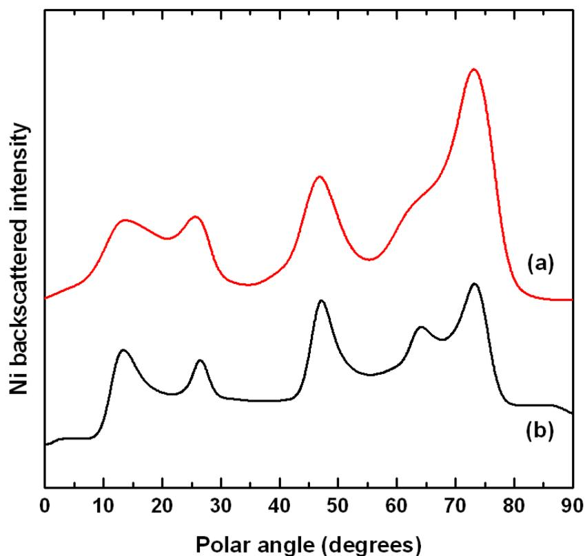
Figure 7.4: (a) Experimental Ni backscattered intensity profile from the Ni(110)-(3×1)-O surface in the  $\langle 100 \rangle$  azimuth, showing peaks corresponding to scattering from the outermost seven layers of the structure. (b) shows the corresponding profile from the FAN simulation of a trial structure containing expansions in the two outermost interlayer spacings relative to the bulk Ni(110) structure.
