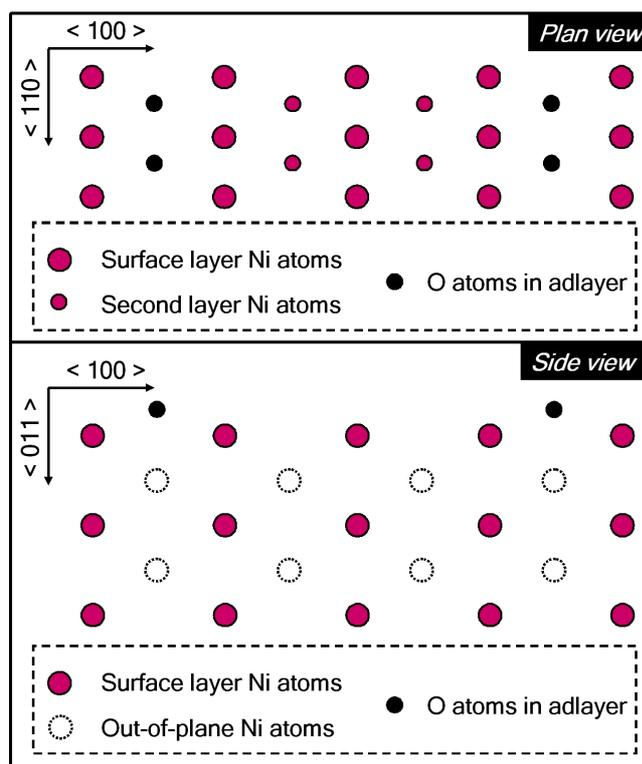
Figure 7.1: A schematic illustration of the  $(3\times 1)\text{-O}$  added row structure formed along rows in the  $\langle 100 \rangle$  direction on the Ni(110) surface. Both the top and side views of the structure are shown.
