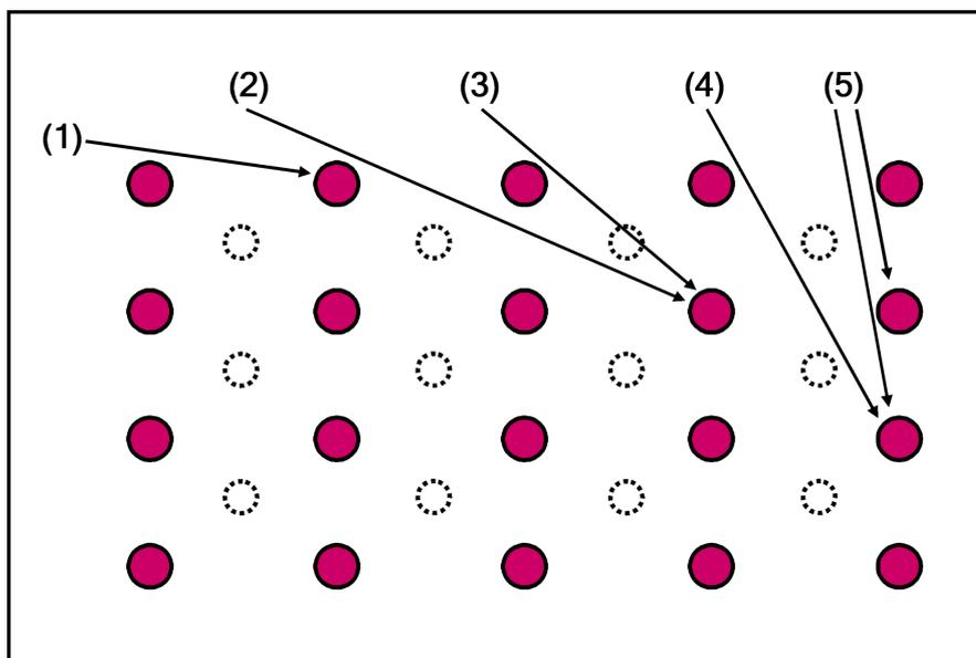
Figure 7.2: The scattering geometries which give rise to peaks in the CAICISS data recorded in the  $\langle 100 \rangle$  azimuth on an f.c.c. (110) surface. Geometries corresponding to odd-numbered layers are shown here, with atoms in these layers represented by the filled circles. The atoms in the even-numbered layers lie in a different plane and are represented by the dashed circles.
