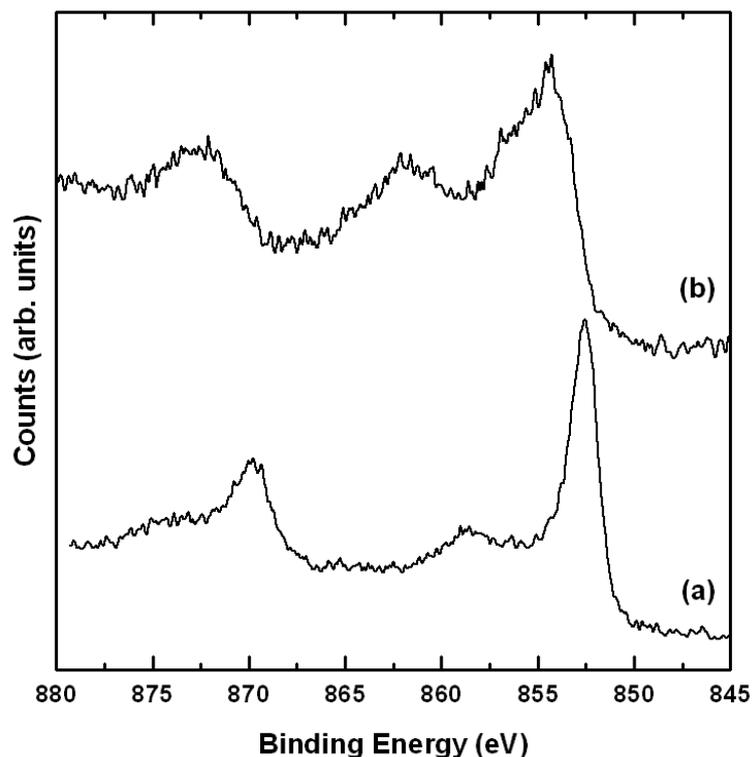
Figure 7.8: The Ni  $2p$  regions recorded from (a) the clean Ni(110) surface and (b) following exposure of the surface to 1800 L of atomic oxygen. Significant chemical shifts and no metallic Ni contributions were observed after oxygen exposure, indicating the formation of a thick NiO film.
