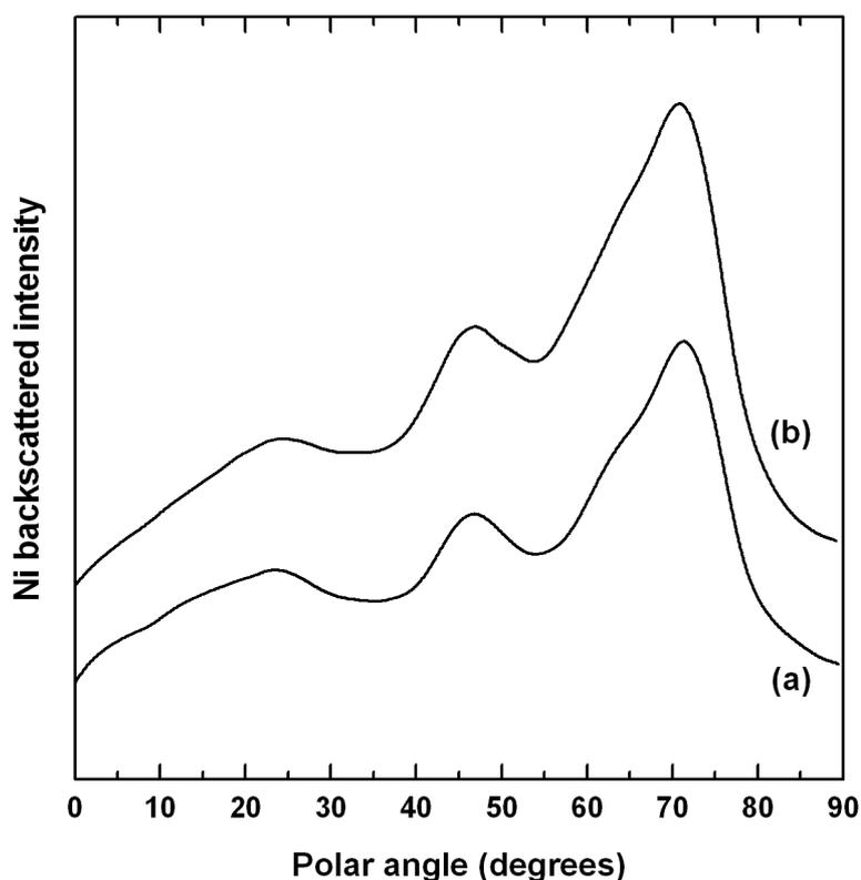
Figure 7.11: The Ni backscattered intensity profiles extracted from the CAICISS data taken (a) prior to and (b) following the deposition of 0.31 ML of Pt on the heavily oxidised Ni(110) surface. No significant changes were observed as a result of the Pt deposition.
