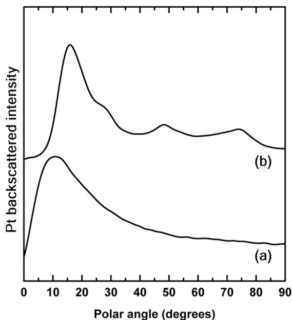
Figure 7.10: (a) The Pt backscattered intensity profile recorded with a 0.31 ML coverage of Pt on the NiO(110) surface. (b) The corresponding data following the deposition of 0.30 ML of Pt on the Ni(110)-(3 $\times$ 1)-O surface, clearly showing a shift in the critical angle and the existence of peaks at higher polar angles associated with the sub-surface Pt atoms.
