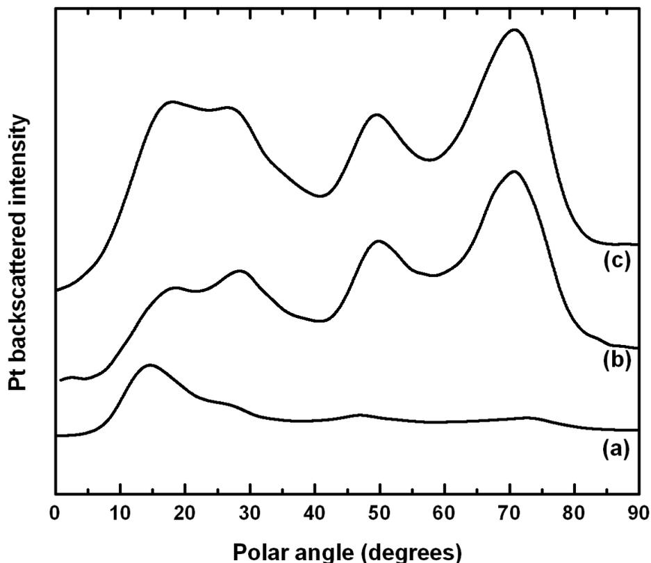
Figure 7.6: The Pt-backscattered profiles extracted from the CAICISS data obtained at Pt coverages of (a) 0.30 ML, (b) 0.88 ML and (c) 1.88 ML on the Ni(110)-(3×1)-O surface. Structural and compositional details are given in the main text and table 7.1.
