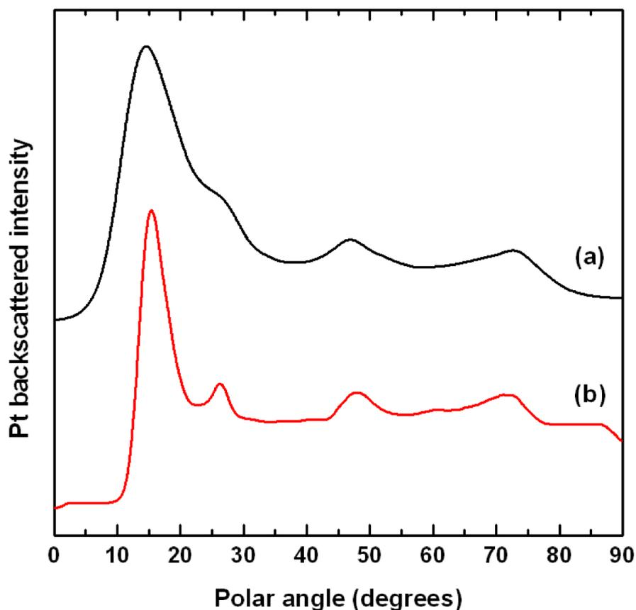
Figure 7.5: (a) The Pt-backscattered intensity profile extracted from the CAICISS data collected in the  $\langle 100 \rangle$  azimuth following the deposition of 0.30 ML of Pt on the clean Ni(110) surface. (b) The simulated Pt profile giving the best fit of these data. The final structure and compositional profile is summarized in table 7.1.
