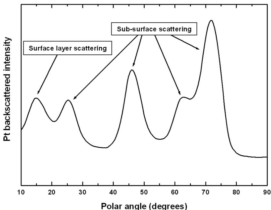
Figure 7.14: The Pt-backscattered intensity profile recorded in the  $\langle 100 \rangle$  azimuth following annealing of a sample containing a 0.80 ML Pt film on top of a NiO(110) surface to 400°C for 10 minutes. The presence of the sharp peaks at polar angles in excess of  $\sim 20^\circ$  indicates a well-ordered structure with a significant amount of Pt atoms which have penetrated into the near-surface region during the annealing process.
