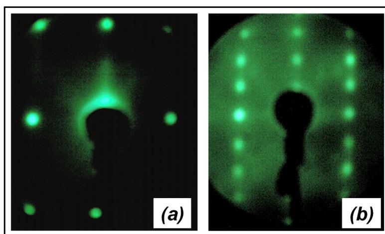
Figure 7.3: LEED patterns observed from (a) the clean Ni(110) surface at 78 eV, and (b) the (3×1) pattern observed at 92 eV following exposure of the clean surface to 1.0 L of atomic oxygen.
