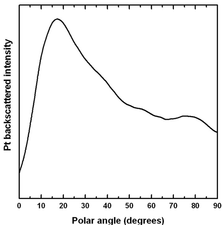
Figure 7.13: The Pt-backscattered intensity profile recorded in the  $\langle 100 \rangle$  azimuth following the deposition of 0.80 ML of Pt on the NiO(110) surface at room temperature. The broad surface peaks arises from the disorder at the NiO(110) surface prior to Pt deposition, whilst the lack of peaks at polar angles in excess of  $\sim 30^\circ$  is indicative of the layer-by-layer growth of a purely Pt film.
