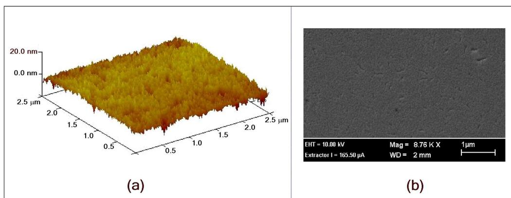
Figure 8.5: (a) AFM and (b) SEM data collected from sample GS1409 (InN(0001)) following the completion of the revised AHC process. Both images show the absence of In droplets on the surface, indicating that this particular AHC has successfully produced a clean, flat, stoichiometric InN surface.
