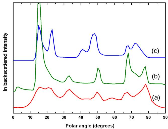
Figure 8.3: (a) CAICISS data collected from sample R799 (InN(000 $\bar{1}$ )) in the  $\langle 1000 \rangle$  direction. (b) shows the corresponding simulation of the bulk InN(000 $\bar{1}$ ) structure (N-polarity), whilst (c) shows the simulation of the bulk InN(0001) structure (In-polarity).
