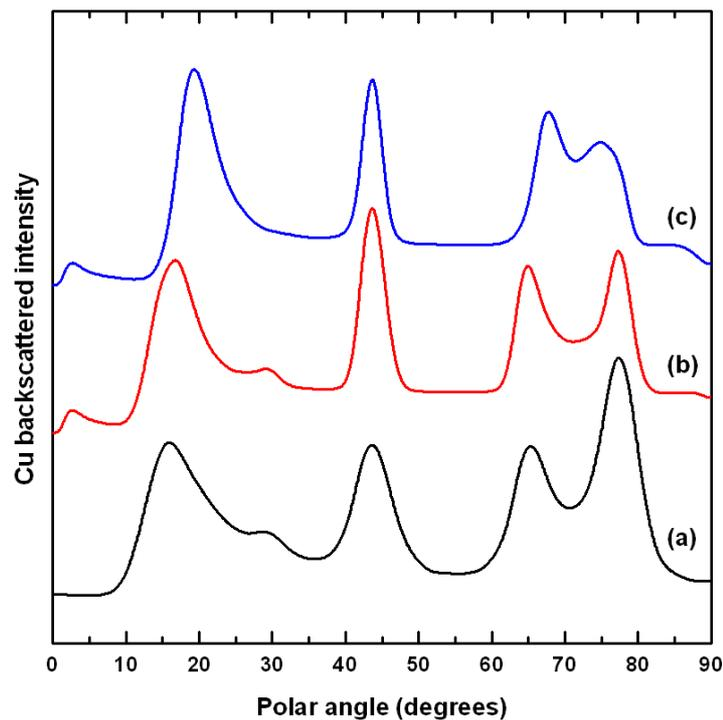
Figure 8.6: (a) The Cu-backscattered intensity profile from the CAICISS data collected in the  $\langle 110 \rangle$  azimuth from the clean Cu(100) surface. (b) The corresponding FAN simulation result using the TFM potential in conjunction with a screening factor of 0.53. (c) The corresponding FAN simulation result using the ZBL potential.
