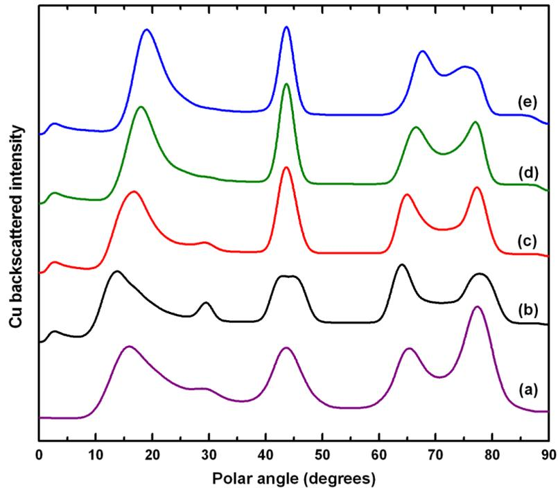
Figure 8.7: (a) The Cu-backscattered intensity profile from the CAICISS data collected in the  $\langle 110 \rangle$  azimuth from the clean Cu(100) surface. Also shown are the corresponding profiles from FAN simulations using the TFM potential with screening factors of (b) 0.40, (c) 0.53, (d) 0.70 and (e) 0.85 (the value calculated from equation 3.9).
