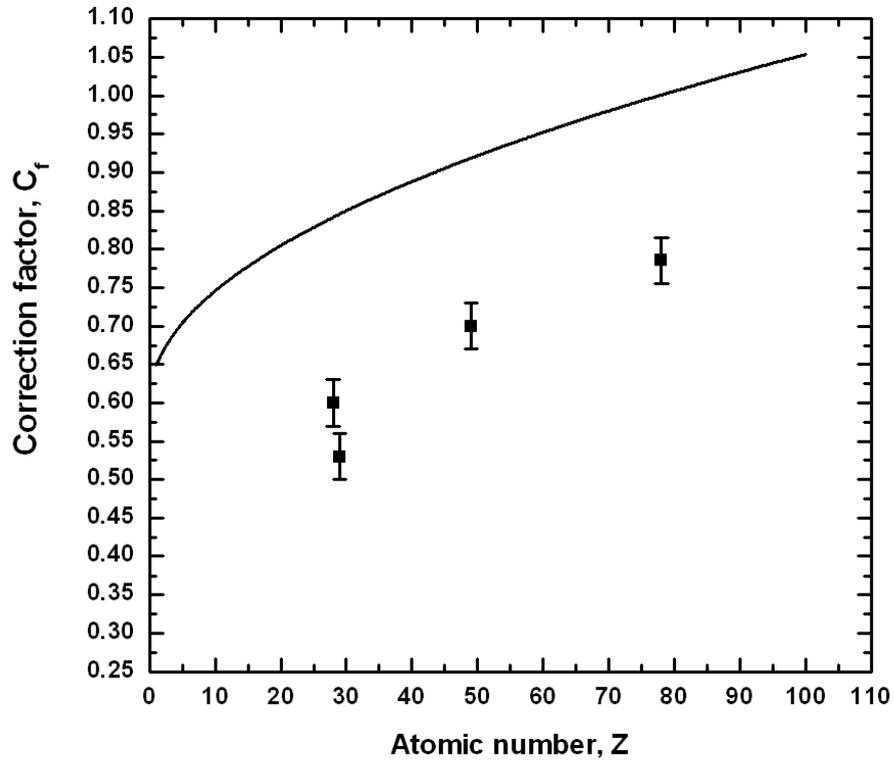
Figure 8.8: The correction factor to the Firsov screening length ( $C_f$ ) as a function of the target atom mass ( $Z$ ), calculated from equation 3.9 (solid line). Also shown are the values determined from CAICISS experiments for Ni, Cu, In and Pt (black squares).
