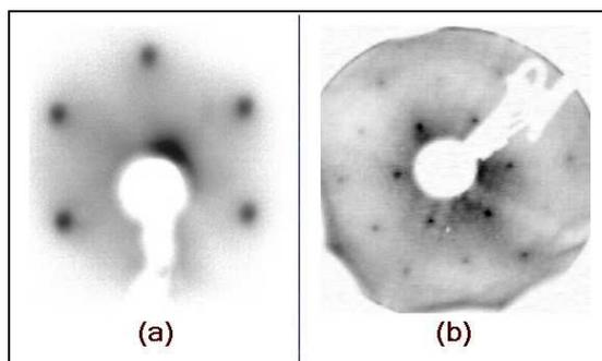
Figure 8.1: LEED patterns recorded following the completion of the AHC process from samples (a) R799 ( $\text{InN}(000\bar{1})$ ) at 79.5 eV and (b) GS1532 ( $\text{InN}(0001)$ ) at 168 eV.
