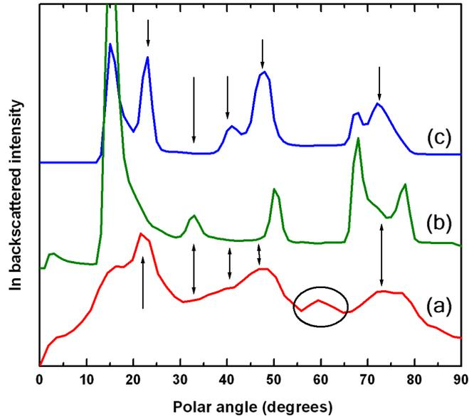
Figure 8.2: (a) CAICISS data collected from sample GS1532 (InN(0001)) in the  $\langle 1000 \rangle$  direction. (b) shows the simulation of the bulk InN(000 $\bar{1}$ ) structure (N-polarity), whilst (c) shows the simulation of the bulk InN(0001) structure (In-polarity). The arrows highlight peaks more accurately described by the In-polarity model, whilst the circled peak at  $59^\circ$  is due to regions of metallic In on the surface.
