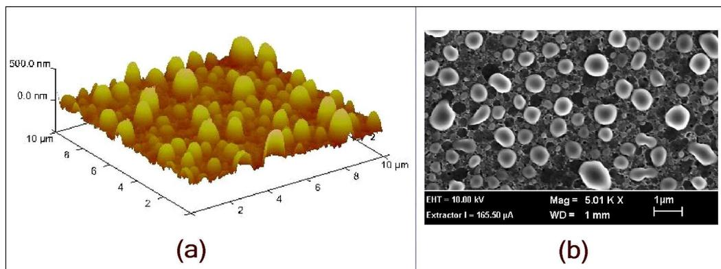
Figure 8.4: (a) AFM and (b) SEM data collected from sample R799 (InN(000 $\bar{1}$ )) following the AHC process. Both images show the formation of large In droplets on the surface, with droplet heights in excess of 200 nm.
