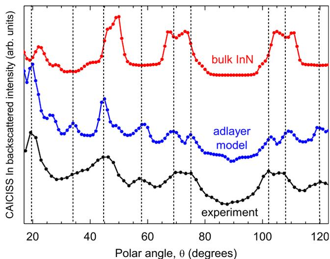
Fig. 1. (Colour online) Experimental CAICISS In-backscattered intensity as a function of polar angle for the [1 0 0] azimuth. Simulated CAICISS spectra are also shown for bulk-like In-terminated In-polarity InN(000 1) and InN(000 1) terminated with In-adlayers, as depicted in Fig. 2.
