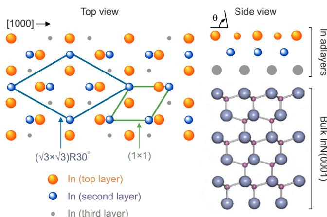
Fig. 2. (Colour online) Structural models showing the top and side views of the In-adlayer surface reconstruction for the In-polarity *c*-plane InN surface. There are three layers of In on top of the In-terminated bulk InN. The topmost layer consists of  $4/3$  ML of In with  $(\sqrt{3} \times \sqrt{3})R30^\circ$  periodicity.
